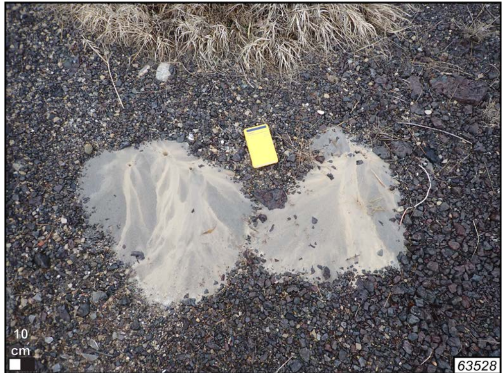
Figure 5. Subaerial sand boils near the I-80/SR-202 interchange and Great Saltair event center. Field notebook (10 cm wide) for scale. Resource ID from the Magna earthquake online clearinghouse labeled in bottom right corner of photo.
