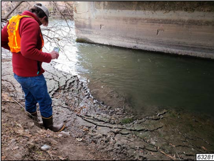
Figure 3. Small, 1 to 2 m lateral spread along the banks of the Jordan River. Resource ID from the Magna earthquake online clearinghouse labeled in bottom right corner of photo.
