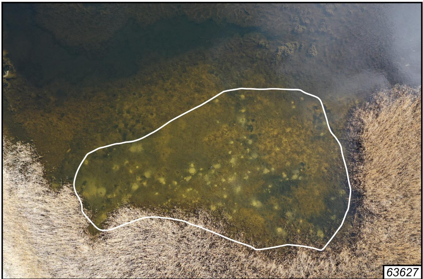
Figure 11. sUAS image of subaqueous sand boils (outlined by white line) near the Great Salt Lake State Park Marina Access Road. Resource ID from the Magna earthquake online clearinghouse labeled in bottom right corner of photo.
