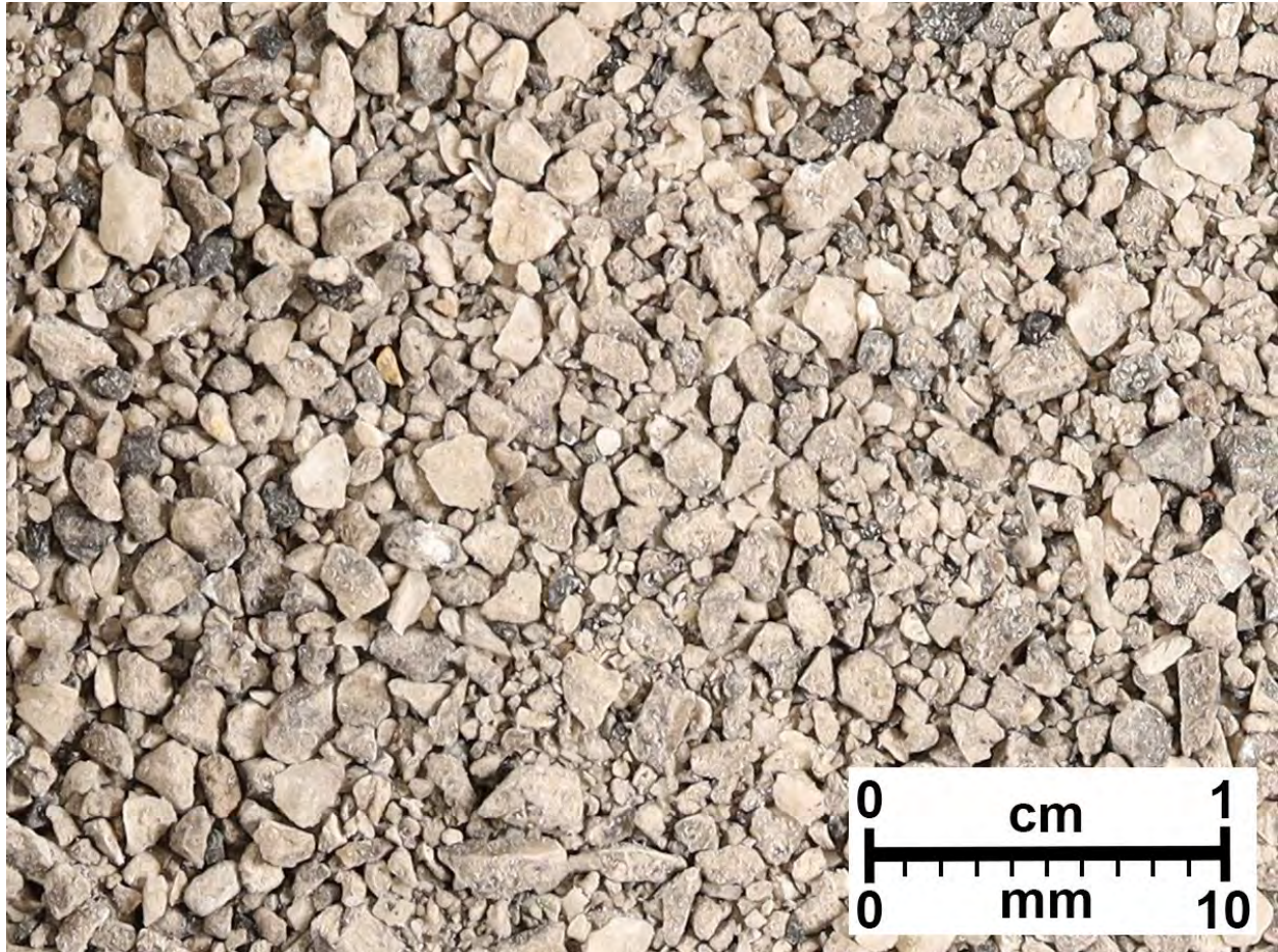
Figure A29. Dolomite, light to dark gray, laminated, argillaceous to shaly in part; shale (10% to 15%), medium to dark gray to black, organic-rich, carbonaceous (sooty); anhydrite (5% to 10%), white, soft to firm, slightly to moderately calcitic.
