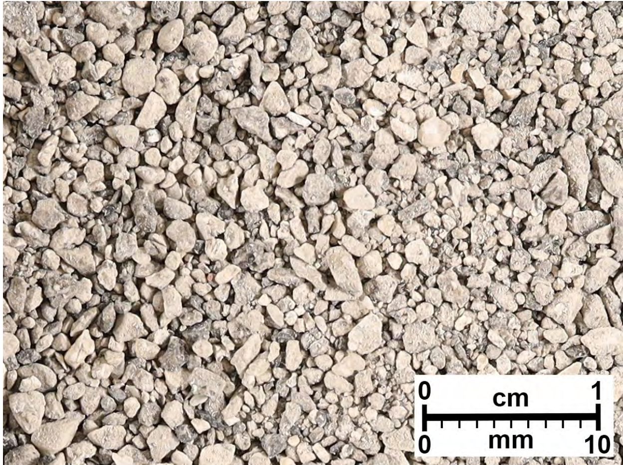
Figure A28. Dolomite, light to dark gray, laminated, argillaceous to shaly; shale (10% to 15%), medium to dark gray, organic-rich, carbonaceous (sooty); anhydrite (5% to 10%), white, soft to firm, slightly to moderately calcitic.
