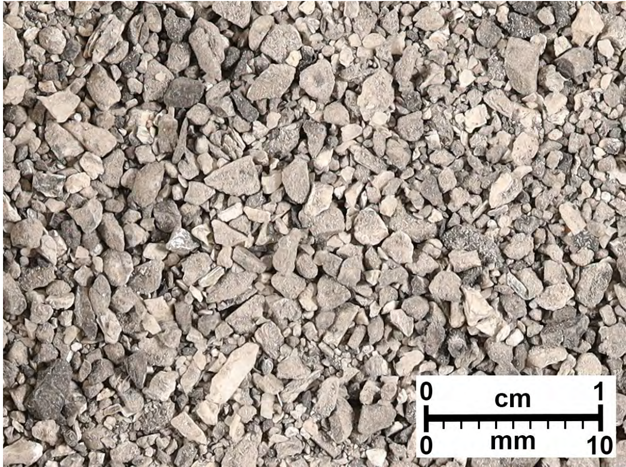
Figure A32. Shale, black to dark gray, soft to firm, organic-rich, carbonaceous (sooty), bitumen, calcareous; dolomite, light to medium gray, chalky to micro sucrosic; anhydrite, light gray to white, soft, chalky; halite.
