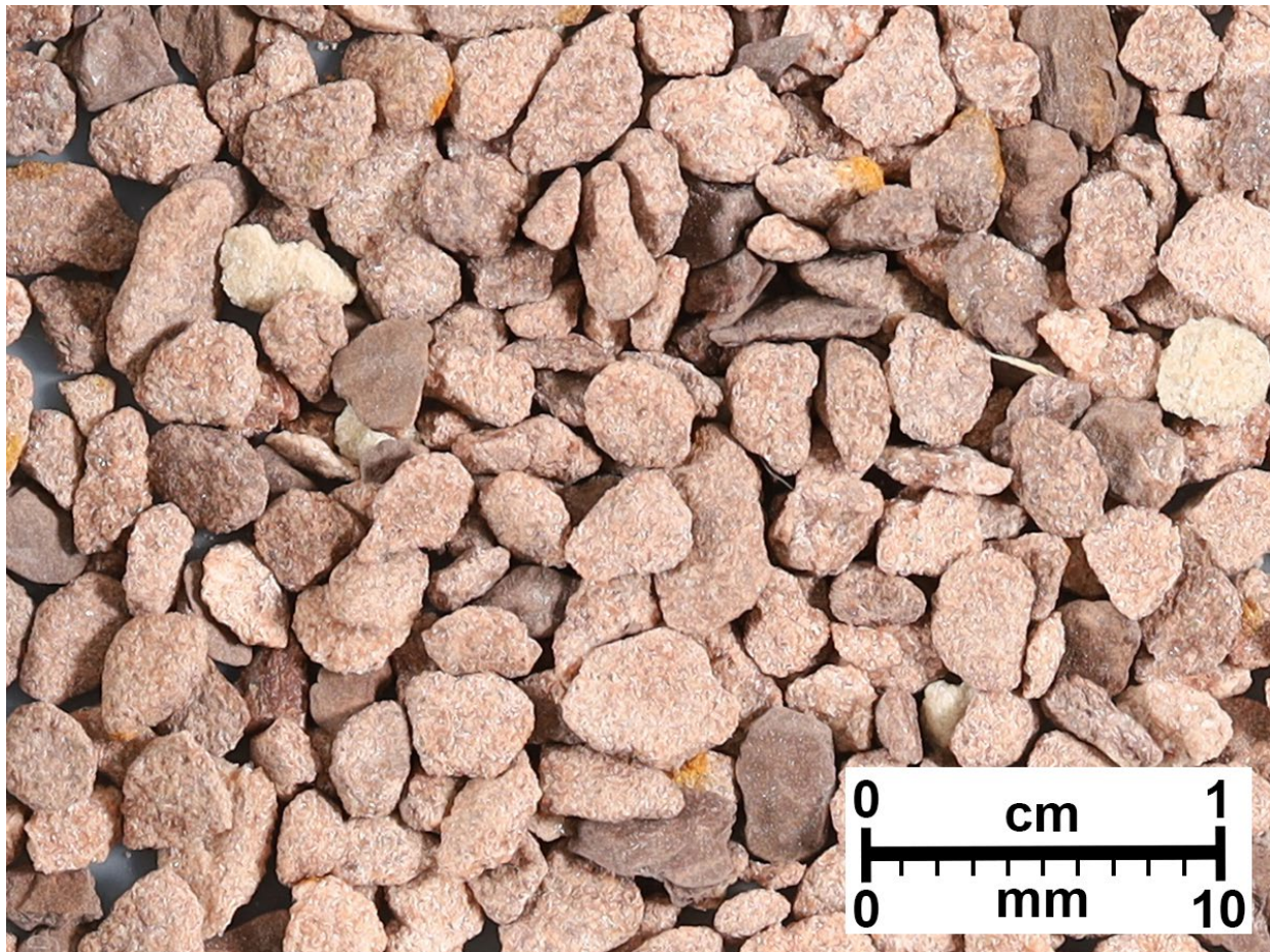
Figure A10. Sandstone, quartzose, pale orange-brown colored, fine grained, friable, well sorted, moderate to good intergranular porosity, siliceous to slightly calcareous cement, occasional red-brown silty matrix.
