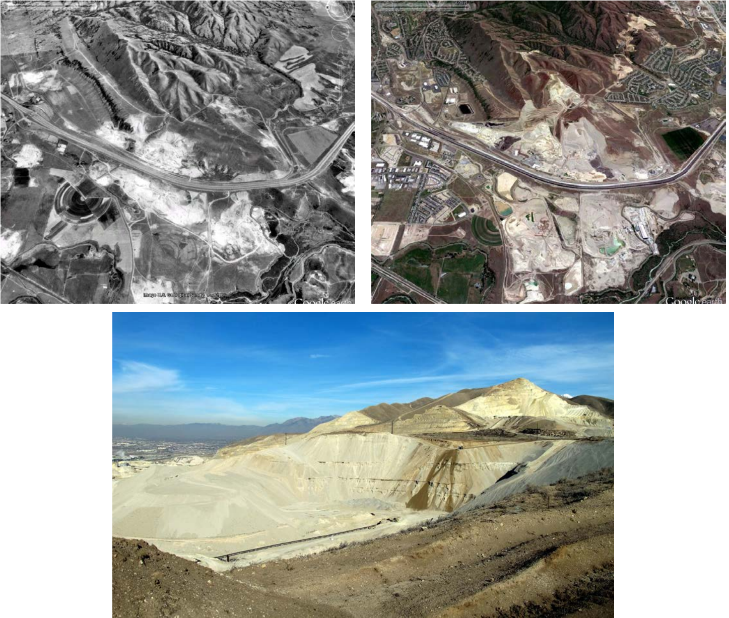
Figure 13. Mining has removed much of the Pleistocene sediments and some of the bedrock at Point of the Mountain. Top photos 1993 (left) and 2015 (right) Google Earth imagery. Bottom photo of gravel pit shows view to the north from Flight Park State Recreation Area in Utah County. Google Earth imagery © 2015 Google Inc.; top left image—U.S. Geological Survey and top right image—Landsat.
