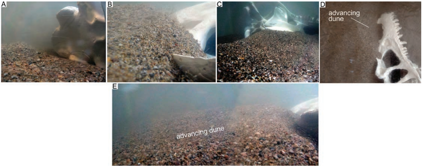
Figure 7. The effects of flow on an Allosaurus skull cast resting on a live-bed of coarse sand. Conditions: sand D_{60} = 0.9 mm, water depth = 20 cm, U = 1 m/s. Overall behavior of the sand is similar to finer grained sand. (A) Scour on upstream side. (B) Burial by advancing dune (streaks in lower right are sand grains in brief suspension). (C) View downstream showing stoss side of advancing dune, skull palate side this time facing upstream; flow stopped for photography. (D) Burial of skull by advancing dune; flow stopped for photography. (E) Profile of advancing dune, skull on right; flow stopped for photography.
