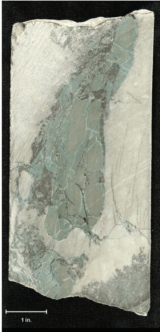
Figure 18. Massive fissure-fill sediments consisting of clay and loessite infiltrated into a large dissolution cavity developed within a well-bedded peloidal/oolitic grainstone. Big Flat No. 3 well (section 23, T. 26 S., R. 19 E., SLBL&M, Grand County, Utah, figure 14), slabbed core from 7677 feet (2340 m).
