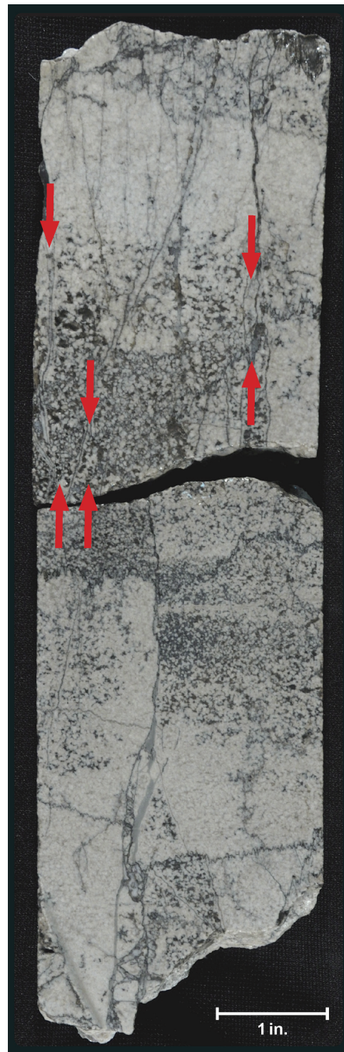
Figure 36. Core slab showing a variety of fracture types, including rimmed microstructures with their distinctive parallel “railroad” or stair-step appearance (see examples between arrows). Long Canyon No. 1 well (figure 14), 7728 feet (2356 m).
