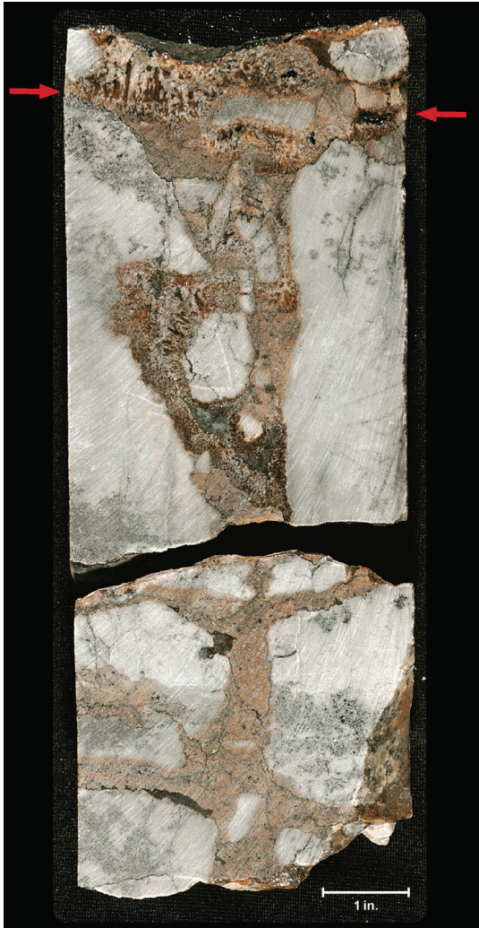
Figure 15. Karst breccia with speleothems (red arrows) capping massive to poorly stratified conglomerate consisting of pink feldspathic sandstone and granitoid clasts between Leadville Limestone country rock. Big Flat No. 2 well (section 11, T. 26 S., R. 19 E., SLBL&M, Grand County, Utah, figure 14), slabbed core from 7729 to 7730 feet (2355.8–2356.1 m).
